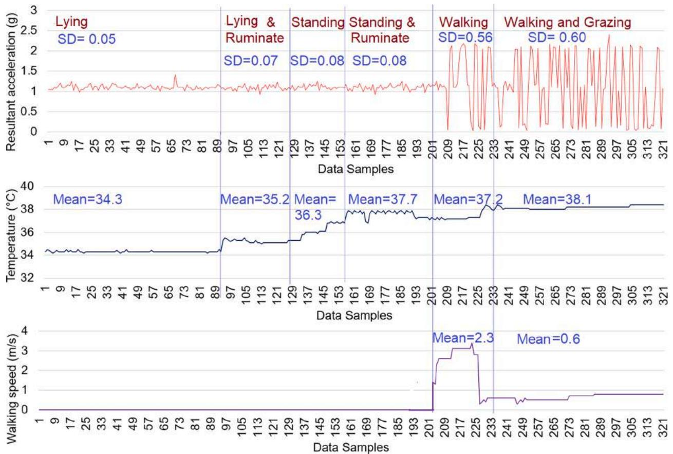
Fig. 6. Raw sensor data profiles concerning all the significant activity states of a cow.
