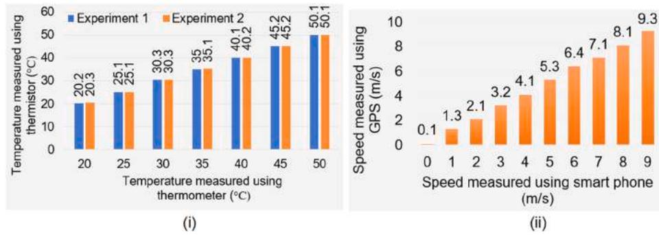
**Fig. 5.** (i) Comparison of temperature measured using thermistor and laboratory thermometer (ii) Comparison of walking speed measured using GPS module and smart phone application.
