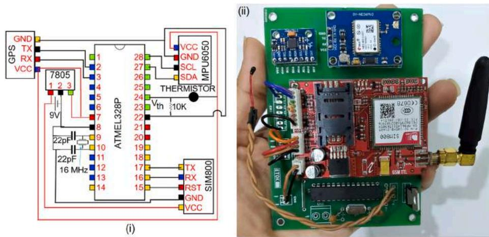
**Fig. 2.** (i) The circuit diagram for the developed device “MOOnitor” (ii) The fabricated PCB assembly for the device.
