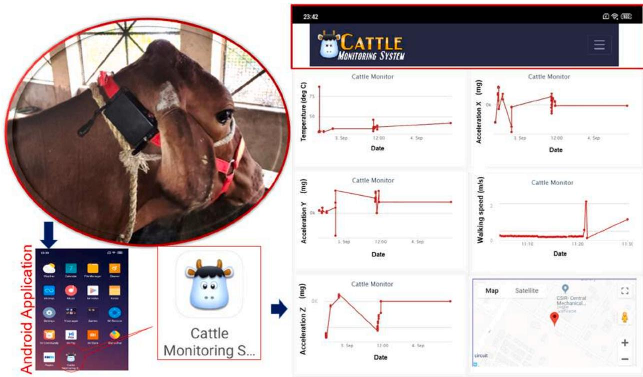
**Fig. 3.** Image depicting the developed device MOOnitor mounted to cattle, the android application and the data seen on smartphone using the android application received in the server.
