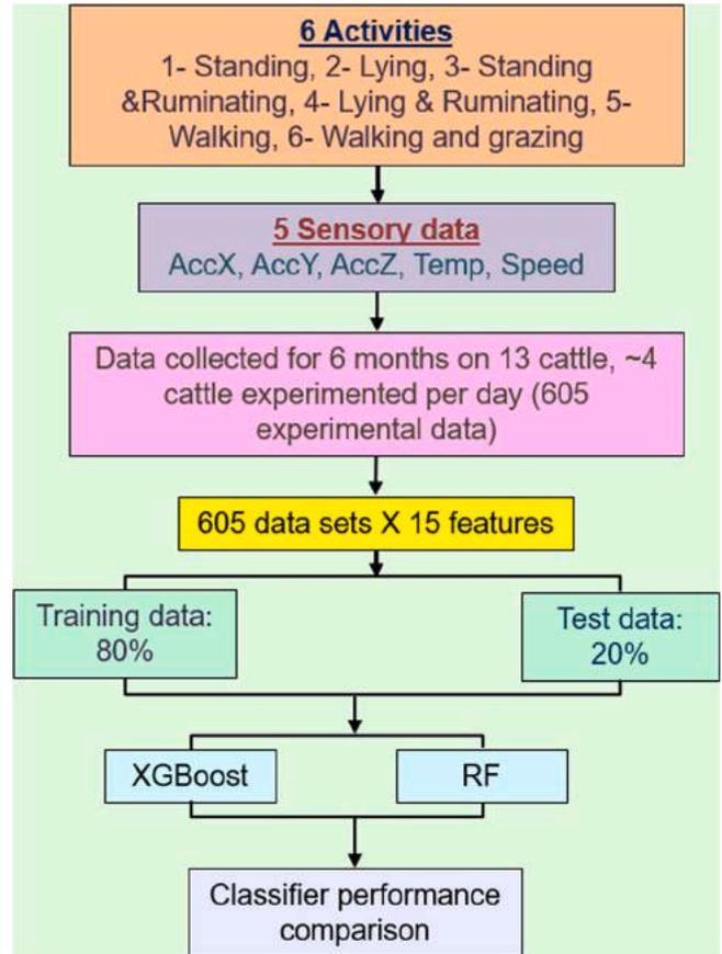
**Fig. 4.** Flowchart for data collection, feature extraction and implementation of classification algorithm.
