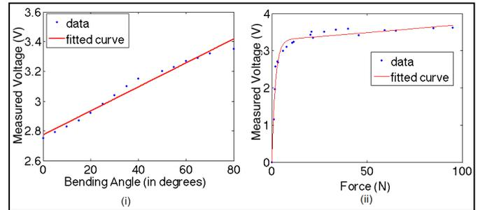
Figure 9: Calibration of- (i) flex sensor using bend angle vs. measured voltage relation and (ii) FSR using force vs. measured voltage relation
