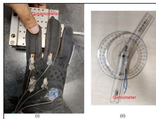
Figure 8: (i) Calibration of an FSR using a force-plate dynamometer (Kistler©, Model no. 9256C); (ii) Calibration of flex sensor using a goniometer.
