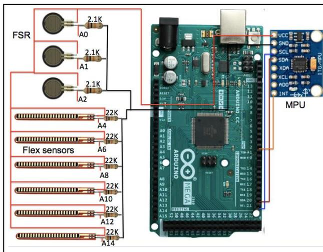
Figure 6: Circuit diagram for connection of flex sensors, FSRs, and accelerometer on an Arduino MEGA platform
