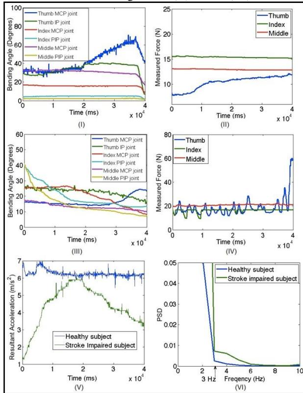
Figure 10: (I) Finger bend angle profile for healthy subject; (II) Finger-tip pressure for healthy subject; (III) Finger bend angle profile for stroke patient; (IV) Finger-tip pressure for stroke patient; (V) Resultant acceleration for healthy subject and stroke patient; (VI) Power spectral density vs. frequency of the acceleration signal for tremor assessment
