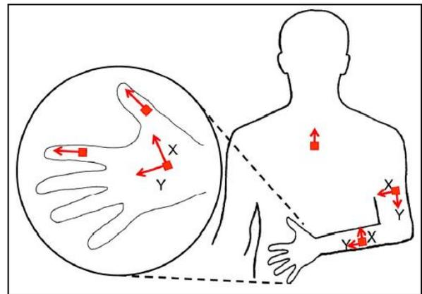
Figure 5: Location of the accelerometer sensors used to monitor human activity (Adapted from [23])
