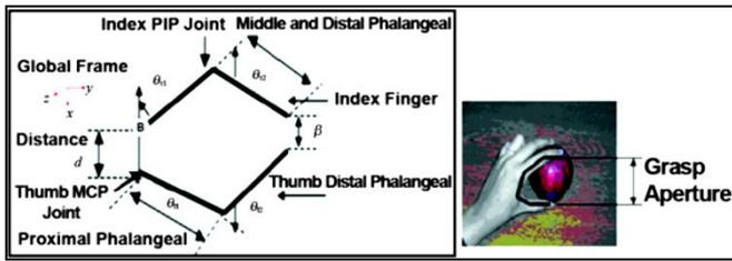
Figure 3: Measurements for instrumented glove used in aperture detection and rehabilitation of stroke patients (Adapted from [24])
