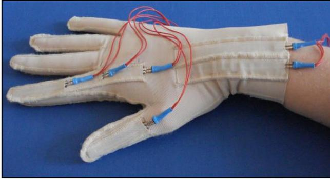
Figure 4: The developed glove for measurement of bending angles of index MCP, PIP, DIP, thumb IP joints and palmar and dorsal flexion of the wrist for diagnosis of stroke affected patients (Adapted from [25])
