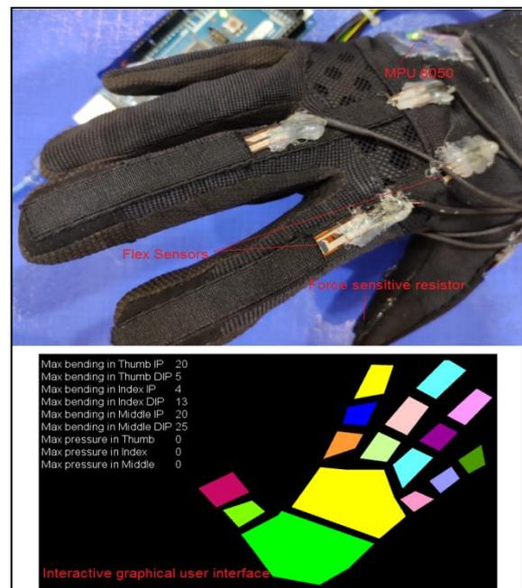
Figure 7: The instrumented glove-based wearable and related processing GUI for stroke diagnosis
