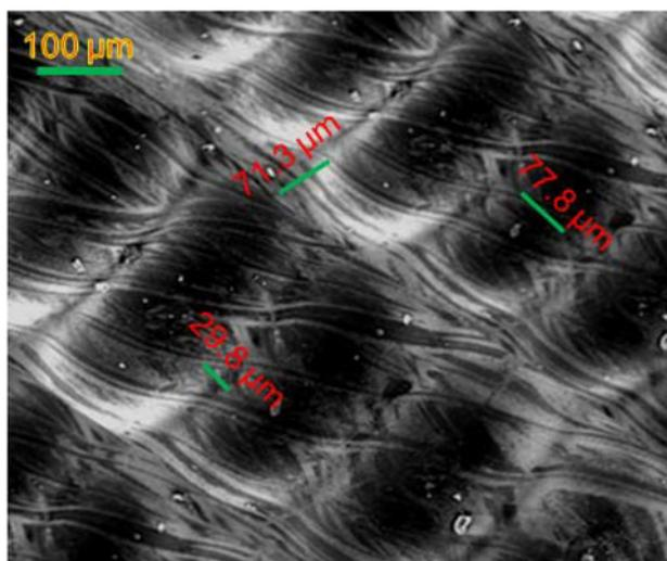
Fig. 2 FESEM image of the developed patterned structures on acrylic using UV laser micromachining
