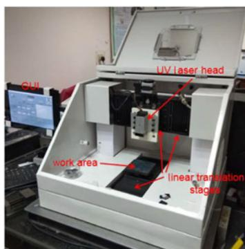
Fig. 1 Experimental setup used for laser micromachining
