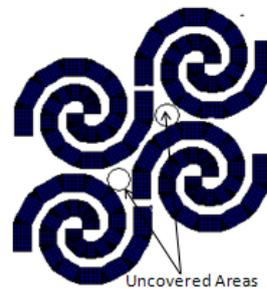
Figure 5. Array of Archimedean spiral antenna
