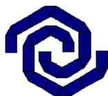
Figure 2. Hexagonal spiral antenna
