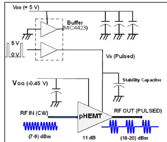
Figure 2. Schematic diagram for drain pulsing
