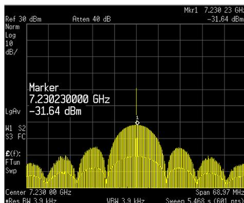
Figure 9. Line spectrum of PPA for 8 dBm input power
