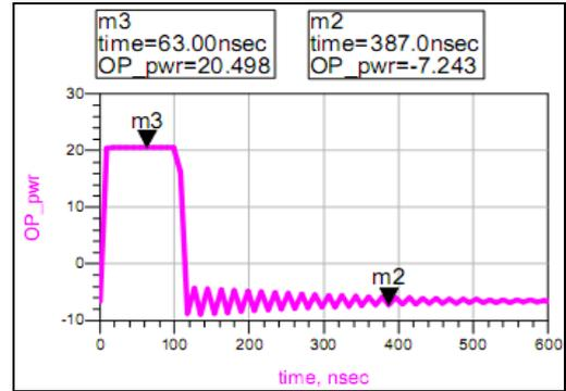
Figure 4. Simulated peak power and leakage power for 9 dBm input drive
