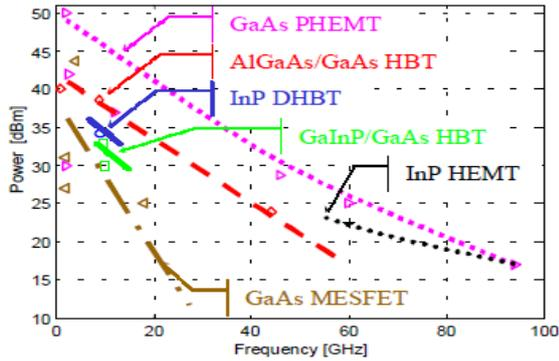
Figure 1. Power performance of MESFETs, HEMTs and HBTs as a function of frequency [5]
