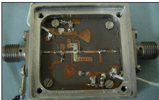
Figure 7. Prototype amplifier housed in Aluminum box
