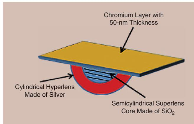
Fig. 5 A schematic for a hybrid superlens with magnification ability.
