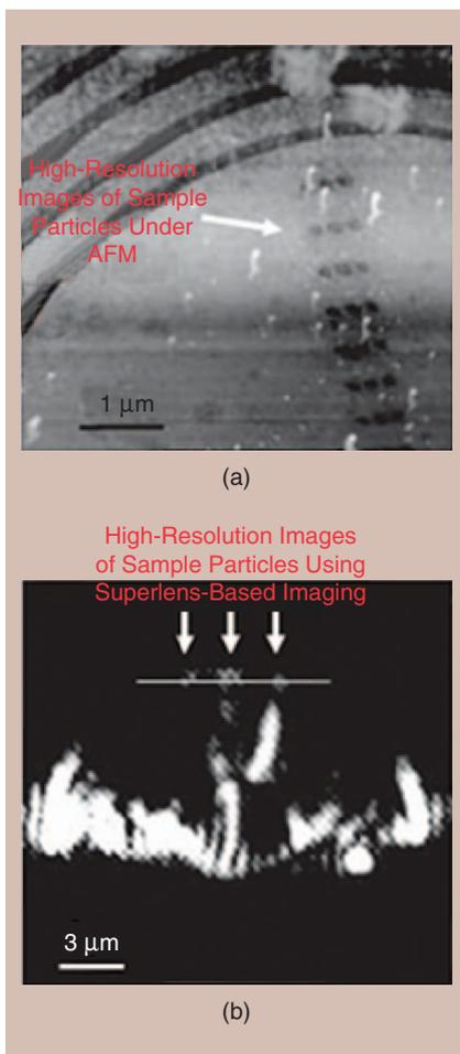
**Fig. 2 (a) A high-resolution image of sample particles under an AFM. (b) High-resolution images of sample particles using superlens-based imaging. (From [I.I. Smolyaninov, Y.J. Hung, and C.C. Davis, "Magnifying superlens in the visible frequency range," *Science*, vol. 315, 2007, pp. 1699–1701]. Reprinted with permission from AAAS.)**
