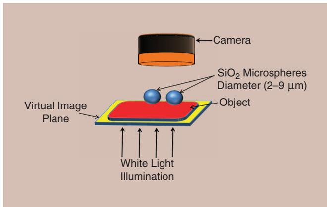
Fig. 4 An optical nanoscope using SiO<sub>2</sub> microspheres.
