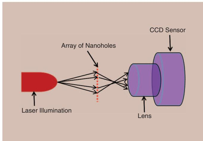
**Fig. 3 Nanoscale imaging using an array of nanoholes.**
