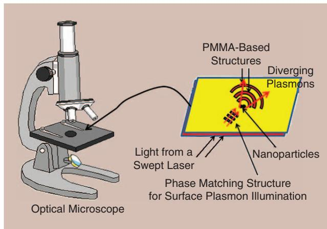
**Fig. 1 The setup for the prototype for nanoscale imaging in the visible frequency range.**
