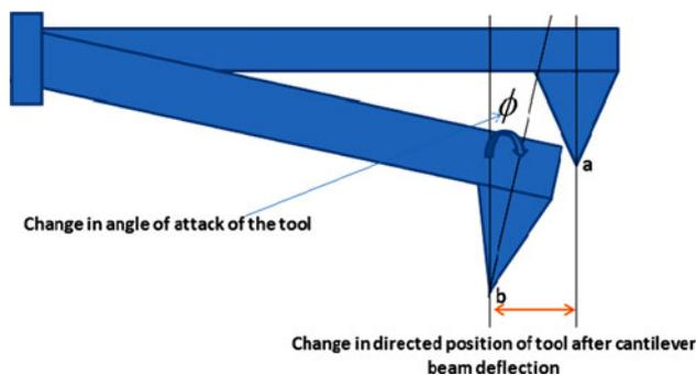
**Fig. 1** Changed tool orientation in AFM based nano-scratching
