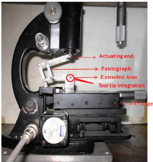
**Fig. 3** Pantograph based micro machine prototype
