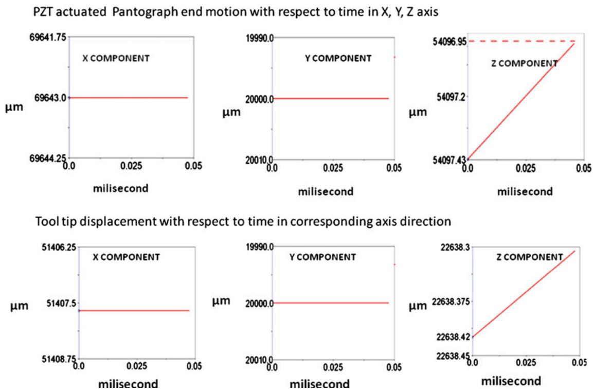
Fig. 9 ADAMS kinematic analysis results for PZT actuators movement and corresponding tool tip movement
