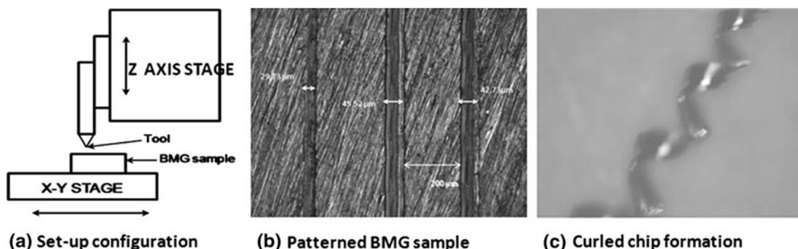
**Fig. 2** Scratching over BMG using a system configured like micro-scale planning
