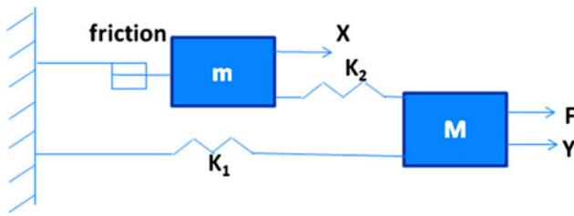
Fig. 7 Dynamic model of linear revolute joint design
