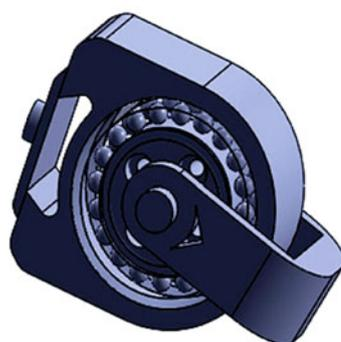
(a) CAD model of Linear revolute joint assembly
