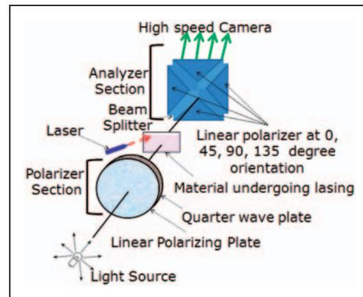
**Figure 1.** Schematic representation of poledioscope design configuration used for dynamic shear stress evaluation.
