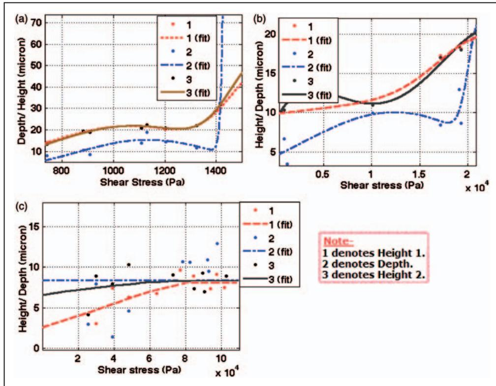
**Figure 4.** Height/Depth vs. shear stress (a) EVA, (b) PMMA and (c) CR-39 (height and depth conventions are as in Figure 3). EVA: ethylene vinyl acetate; PMMA: poly methyl methacrylate; CR-39: ally diglycol carbonate.
