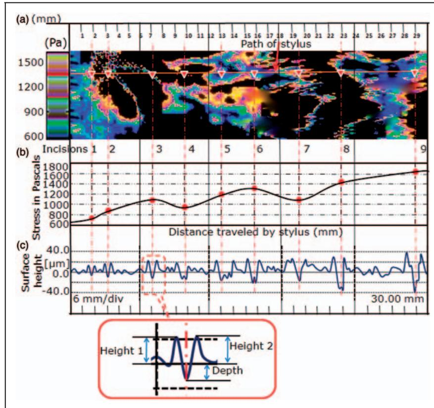
**Figure 3.** (a) Reconstructed shear stress map for EVA sample, (b) shear stress magnitude at the intersection of stylus and laser point and (c) waviness (W) profile of lasered EVA.
