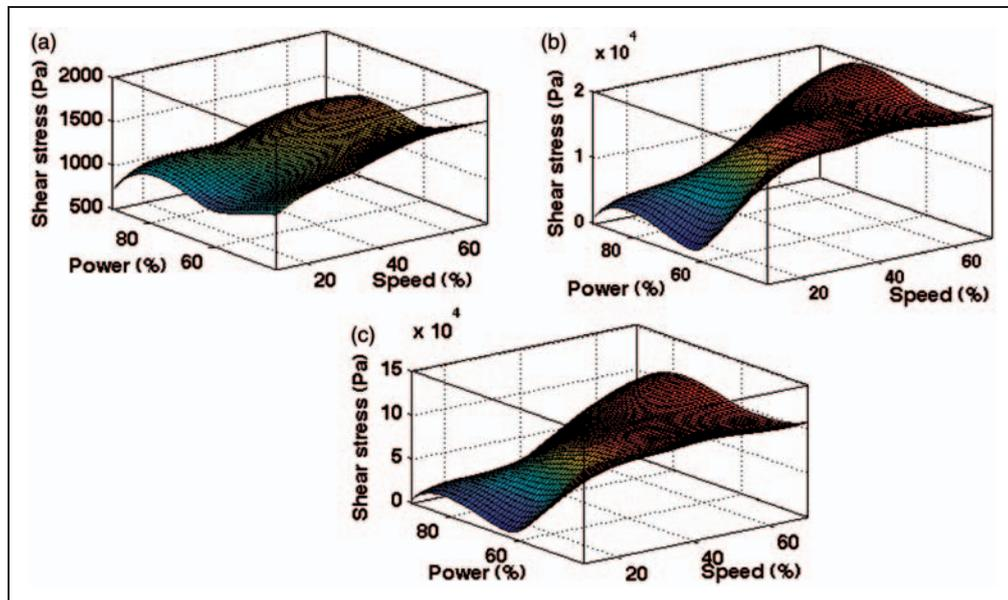
**Figure 5.** Surface plots for variation of shear stress with power and speed (a) EVA (b) PMMA (c) CR-39. EVA: ethylene vinyl acetate; PMMA: poly methyl methacrylate; CR-39: ally diglycol carbonate.
