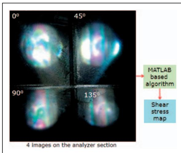
**Figure 2.** Four images obtained from analyzer section showing induced birefringence due to thermal stress.
